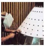
Weld-on Winco Surf high alumina ceramic tiles protect Alloys can be placed with this cone against wear and thermal shock.
