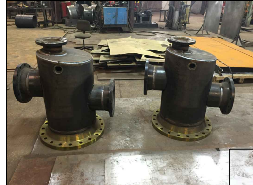
RECIRC TANK STRAINER HOUSINGS
