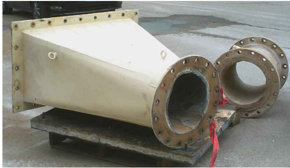
Champaloy Lined Lime Stone Chute
