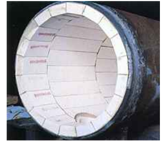
Ceramic Lined Pipe Fabrication
