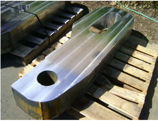
Furnace Pusher Fingers
