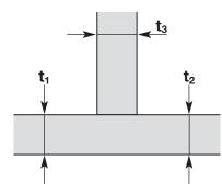
Combined Plate Thickness: T Joint  $t = t_1 + t_2 + t_3$ Butt Joint  $t_3 = 0$
