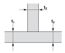
Combined Plate Thickness: T Joint  $t = t_1 + t_2 + t_3$ Butt Joint  $t_3 = 0$
